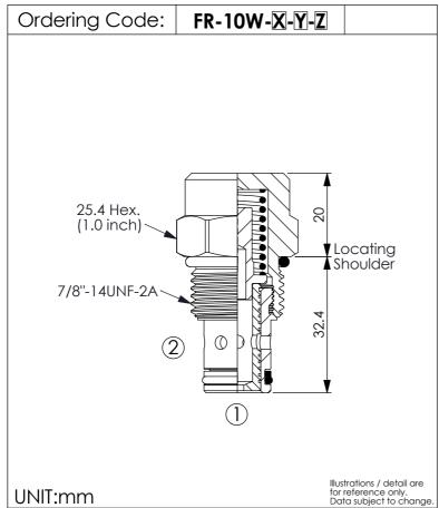
**TECHNICAL DATA** 240 Max. pressure: bar 23 Rated Flow: I/min 10W-2 Cavity-Tooling: Installation torque: 35 - 45 Nm
