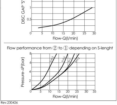
Performance curves R/flow (allowance can be ±10% from the curve) After assembling the valves are preadjustated at the following valves "S"= 0.7 mm
