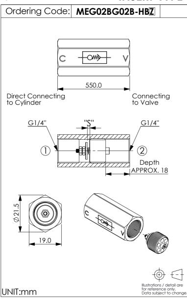
Hose burst Hose burst valve check valve with orifice
