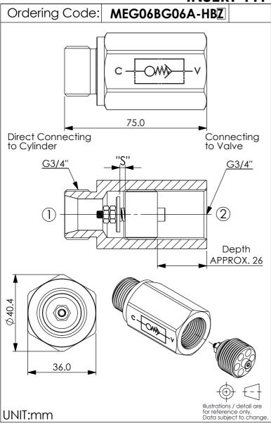
Performance curves R/flow (allowance can be  $\pm 10\%$  from the curve) After assembling the valves are preadjustated at the following valves "\$"= 2.8 mm
