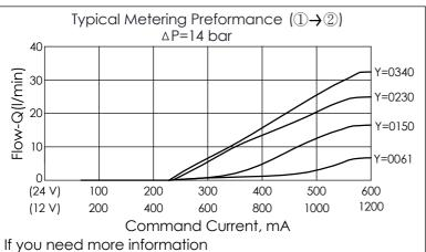
Note: Flow in the @to@direction is limited to about 5 LPM
