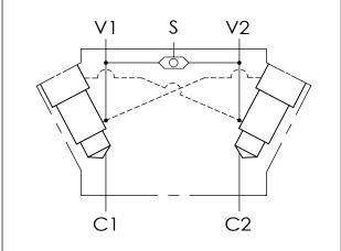
**TECHNICAL DATA** Aluminum (A41) Body Pressure Rating: 210 bar Ductile Iron(\$41) 350 bar Body Pressure Rating:
