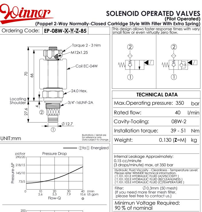
Coils must be ordered separately Mounting Position: unrestricted X **STRUCTURE**
