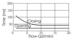
The performance curve or data is only for reference, as customers' using condition, pressure, flow, hydraulic fluid viscosity, cleanliness, temperature and so on are different, the curve or data will be
