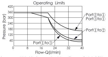
he performance curve or data is only for reference, as customers' using condition, pressure, flow, hydraulic fluid iscosity, cleanliness, temperature and so on are different, the curve or data will be different.
